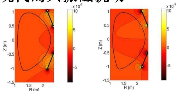
Figure 3.1: Poloidal cuts (in the plane  $\varphi = 30^\circ$ , which approximately corresponds to the middle of a coil) of  $B^R$  (left) and  $B^Z$  (right) produced by the I-coils fed with 1kAt, in Teslas. The I-coils appear as black bars, and the plasma separatrix is also represented.
