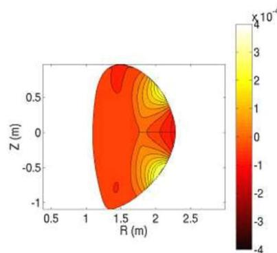
Figure 3.2: Poloidal cut (in the plane  $\varphi = 30^\circ$ , as in 3.1) of  $b^r$  (dimensionless quantity) produced by the I-coils in even parity configuration fed with 1kAt.
